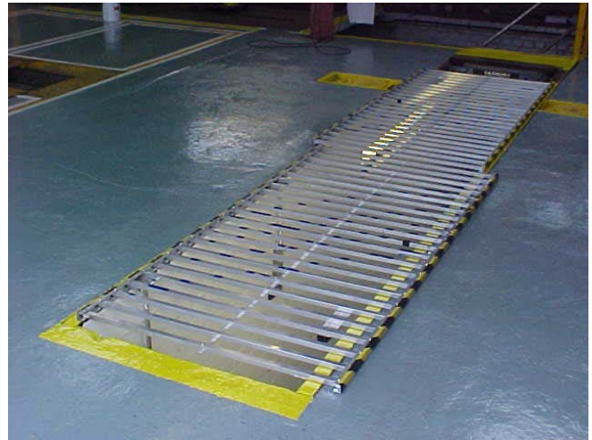
CAVE system in position over a vehicle inspection pit; protecting technicians and visitors from exposed void
